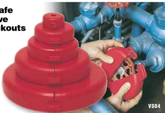
Helps to properly lockout valve handles from 1" up to 14" diameter. Designed with (2) flattened half-moons that completely cover valve wheel. Made from polypropylene plastic. Fully dielectric and resistant to extreme temperature changes (-50° F to 360° F). Resistant to cracking and abrasion. Meets OSHA 29 CFR 1910.147 regulations and ANSI Z353.1. Red.
